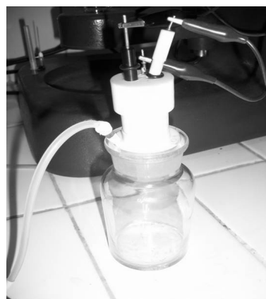
Figure 2. Three-electrode system of the electrochemical cell placed in the sealed glass container
