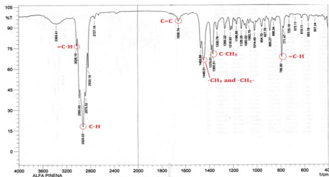
Figure 2. FT-IR Spectrum of Turpentine Oil Distillate
